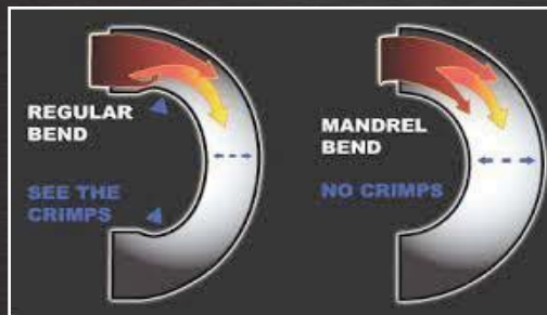
Figure 1.2 The difference between mandrel and empty bends.
