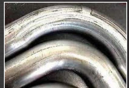
Figure 1.4 Difference between mandrel and empty bends.
